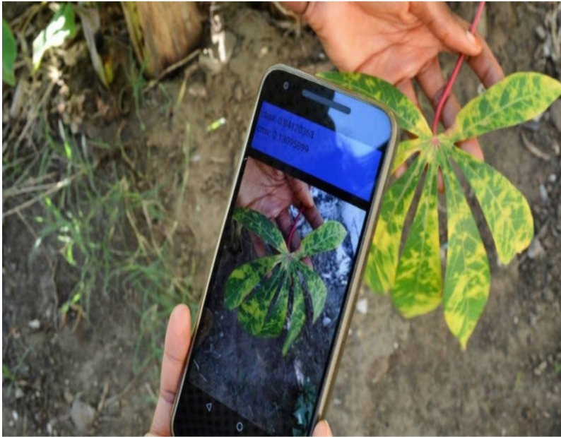
Plant disease classification with TensorFlow Lite on Android
